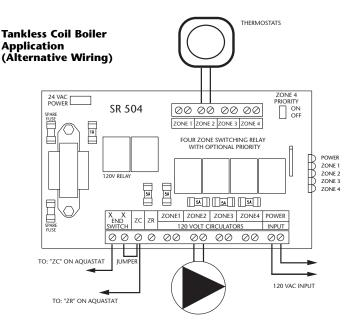
**Operation:** When any thermostat calls for heat, the boiler is given a signal to start. The appropriate circulator is energized only when the boiler temperature is above the set low limit.
