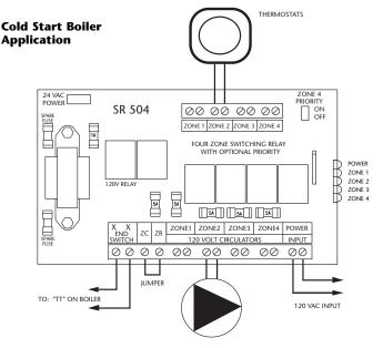
**Operation:** When any thermostat calls for heat, the appropriate circulator is energized and the isolated end switch (X and X) will start the boiler.
