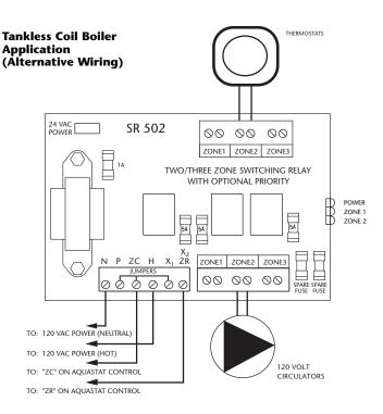
**Operation:** When any thermostat calls for heat, the boiler is given a signal to start. The appropriate circulator is energized only when the boiler temperature is above the set low limit.
