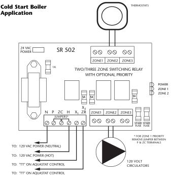
**Operation:** When the thermostat calls for heat, the appropriate circulator is energized and the isolated end switch  $(X_1 \text{ and } X_2)$  will start the boiler.
